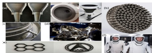
Fig 7. (a) The constructed views of the antenna prototype show the antenna construction as (a) made and coated half sections and assembled. [62] (b) EOS produced a baseplate with an all-in-one design for Inconel 718 printing utilizing selective laser melting (SLM), (c) Flex joint of the RS-25 [63] (d) the SuperDraco engine from SpaceX [64] (e) Chinese satellites carried two examples of continuous fiber-reinforced 3D printed parts: a honeycomb structure and a logo for China Aerospace Science and Technology Group Co., Ltd. [65] (f) gradient background for a SpaceX suit 3-D IMPRESSION HELMET The 3-D printed helmet's personalized padding provides valves that control the pressure systems in the suit as well as microphones for communication. Doug Hurley and Bob Behnken in their SpaceX spacesuits [66].
